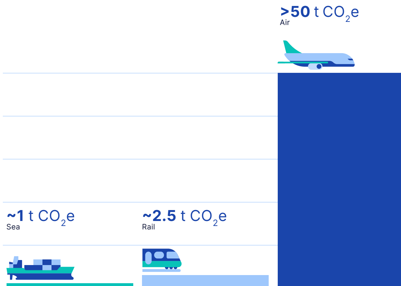
Average emissions of shipping one 20 ft container (10 tons of freight) from Far East Asia to Northern Europe
